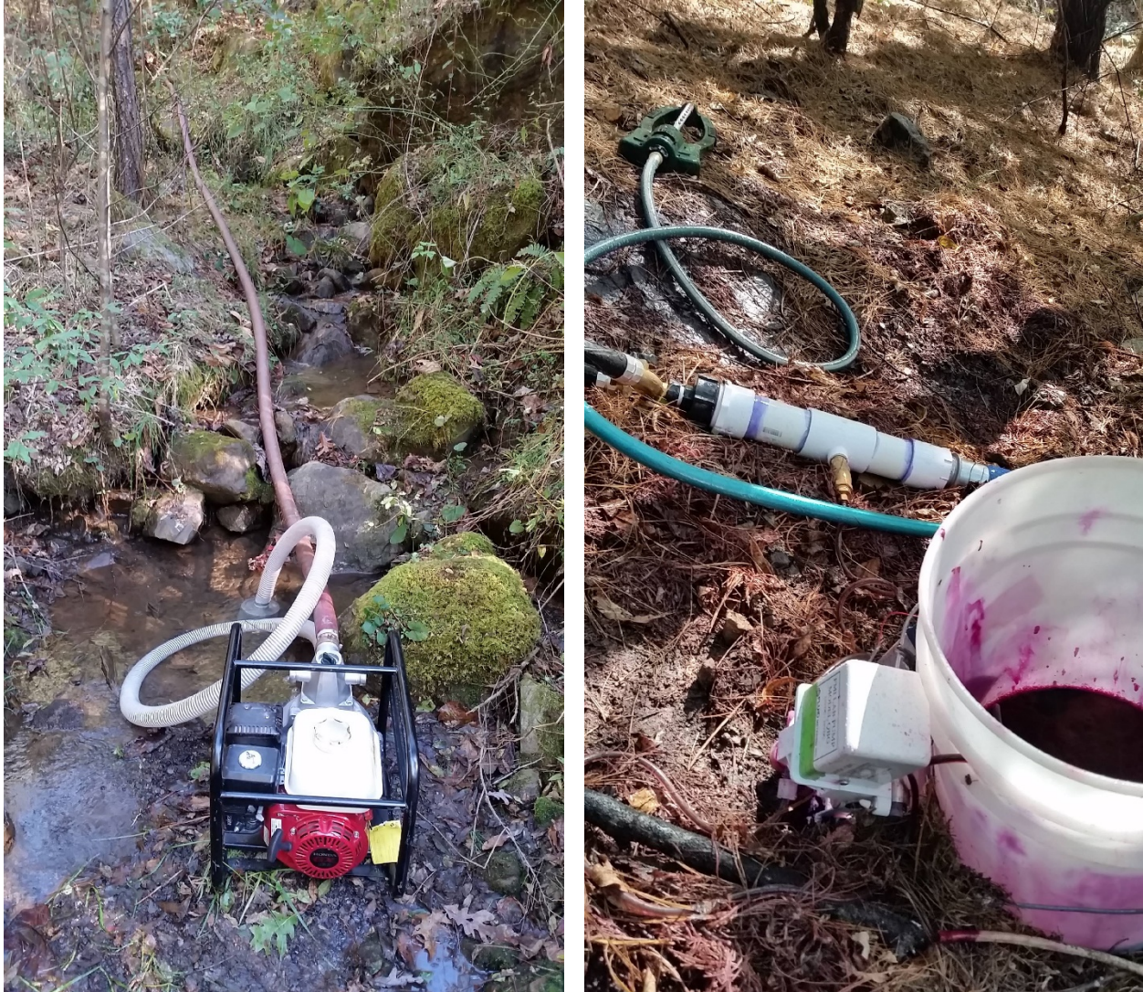
Figure 3-3. Water pump (left) and rhodamine WT injection and sprinkling system (right) used in artificial rainfall with tracer experiments in August and October 2017.
