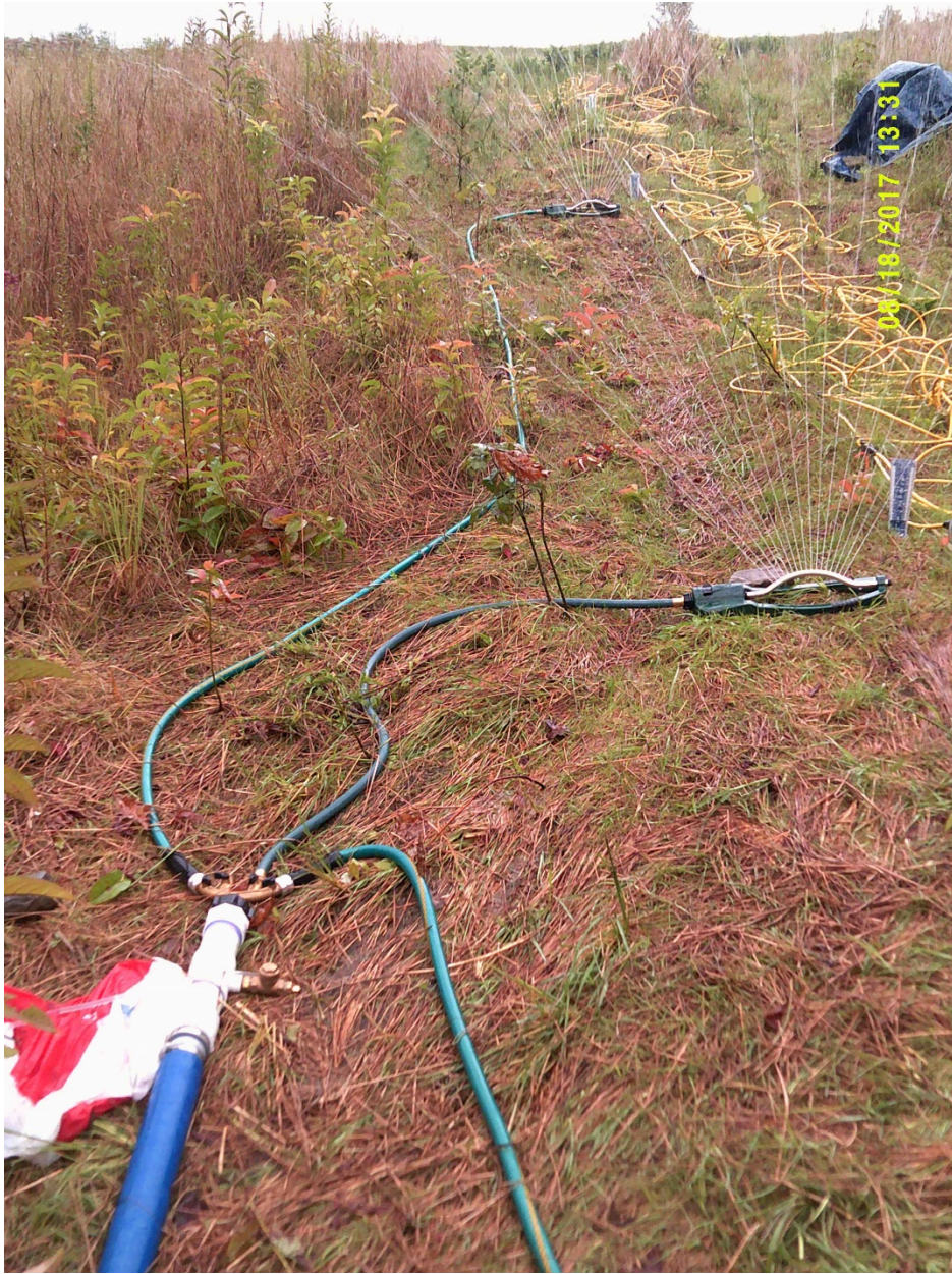
Figure A-7: Garden Hose and Sprinkler Setup
