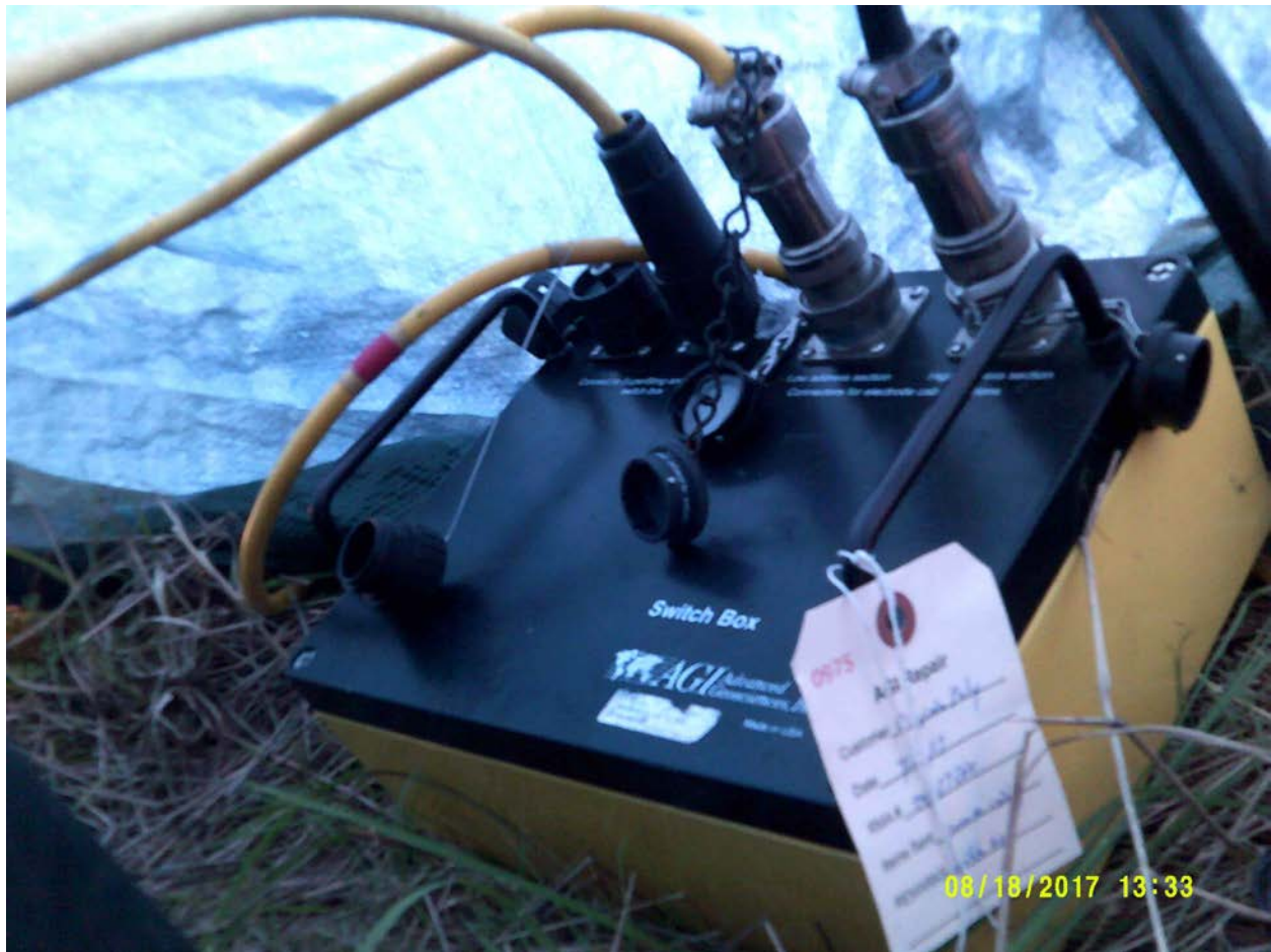
Figure A-2: Switch Box Setup
