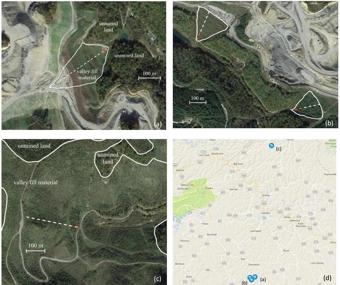
Figure 3-1. Aerial view of the four field sites: (a) Barton Hollow; (b) Office Fill (top left) and End Fill (bottom right); (c) Bearwallow. White solid lines denote the approximate location of fill boundaries. The Bearwallow fill was constructed within a mined landscape and therefore does not have clearly defined perimeter boundaries as do the other three fills. White dashed lines denote the locations of long ERI transects. Red dashed lines denote the locations of short ERI transects with artificial rainfall. Areal map (d) shows the relative locations of the four sites. All views are oriented such that north is up.
