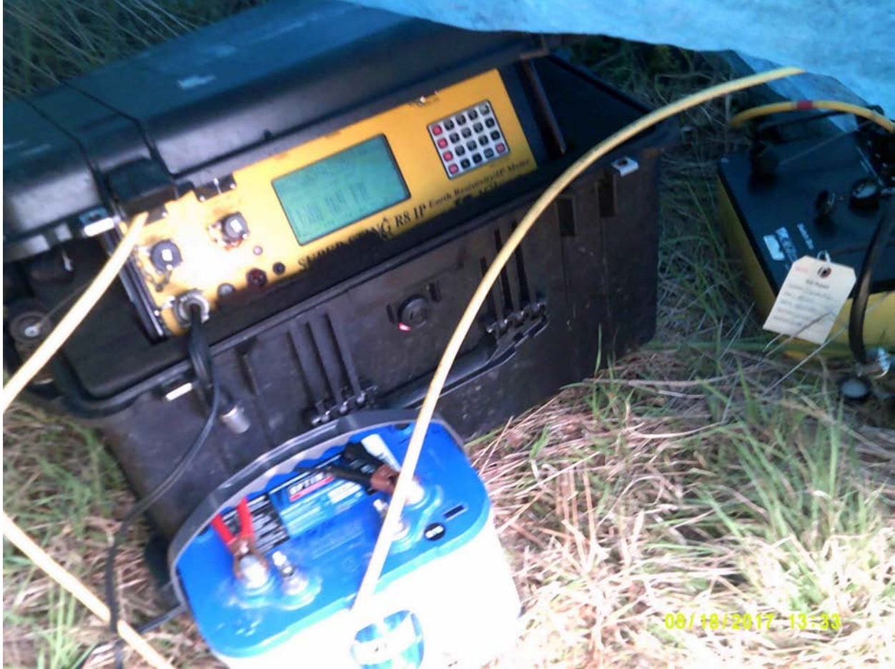
Figure A-3: Resistivity Meter Setup The resistivity meter is connected to the switch box (right) and the marine battery (front).
