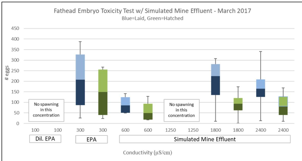
**Figure 26.** Fathead minnow egg and embryo toxicity testing of simulated mine effluent.
