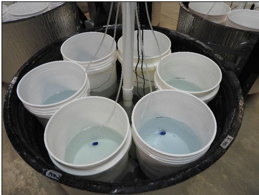
**Figure 3.** Each of the six randomly placed concentrations in one of the four water baths. Each bucket has 10 liters of test water and an airstone. This is a close-up picture of a water bath with six 5-gallon buckets filled with 10 liters of water.
