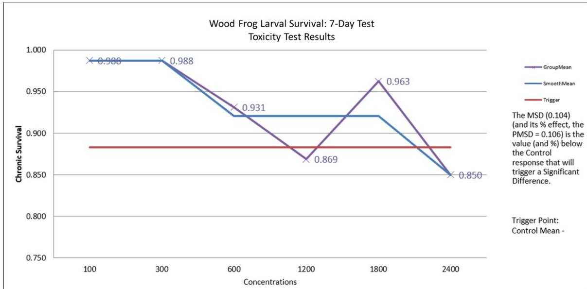
**Figure 20.** Wood frog larvae survival during a 7-day conductivity toxicity test (NOEC = 1,800  $\mu\text{S/cm}$ ; LOEC = 2,400  $\mu\text{S/cm}$ ).
