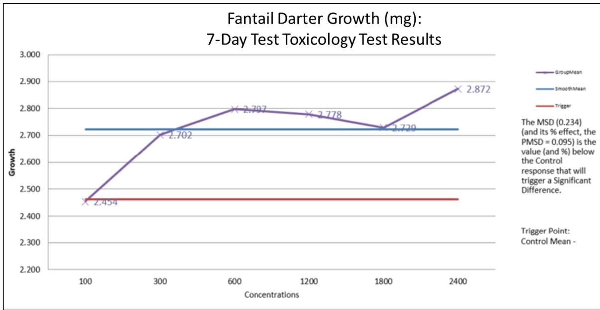
**Figure 25.** Fantail Darter larval growth (mg) of a 7-day conductivity toxicity test with a LOEC of  $> 2,400 \mu\text{S/cm}$ .
