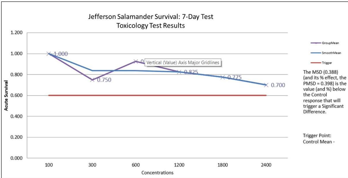
**Figure 22.** Jefferson salamander larvae survival during a 7-day conductivity toxicity test with a NOEC of 1,800  $\mu\text{S}/\text{cm}$  and LOEC of 2,400  $\mu\text{S}/\text{cm}$ .
