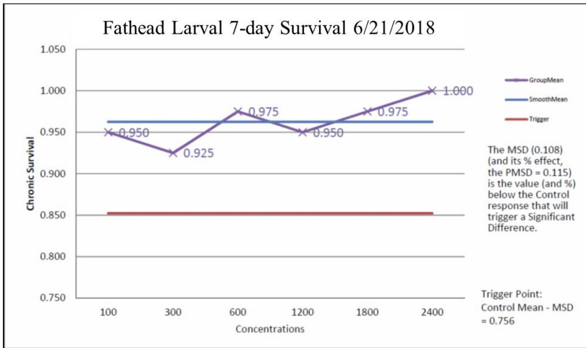
**Figure 27.** Results from the fathead minnow larval 7-day chronic survival testing showed an NOEC of 2,400  $\mu\text{S/cm}$ , a LOEC >2,400  $\mu\text{S/cm}$  and an EC25 >2,400  $\mu\text{S/cm}$ .
