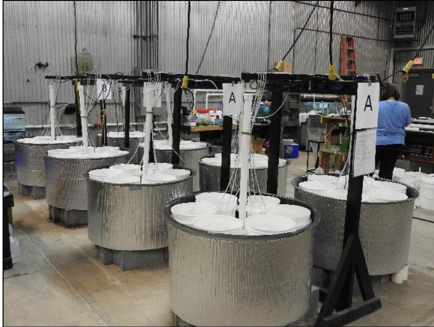
**Figure 2.** Toxicological testing set-up at Virginia Tech. This picture shows eight 50-gallon water baths with six 5-gallon buckets in each water bath.
