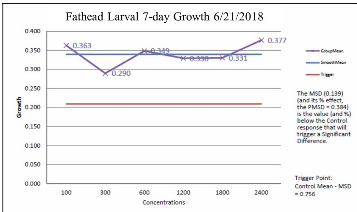
**Figure 28.** Fathead minnow growth was also analyzed during this 7-day test. Results showed an NOEC of 2,400  $\mu\text{S/cm}$ , a LOEC >2,400  $\mu\text{S/cm}$  and an IC25 >2,400  $\mu\text{S/cm}$ .
