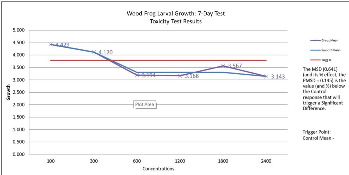
**Figure 21.** Wood frog larvae growth (in milligrams) during a 7-day conductivity toxicity test. Wood frog tadpole growth exhibited a significant decrease with a NOEC of 300  $\mu\text{S/cm}$  and a LOEC of 600  $\mu\text{S/cm}$ .
