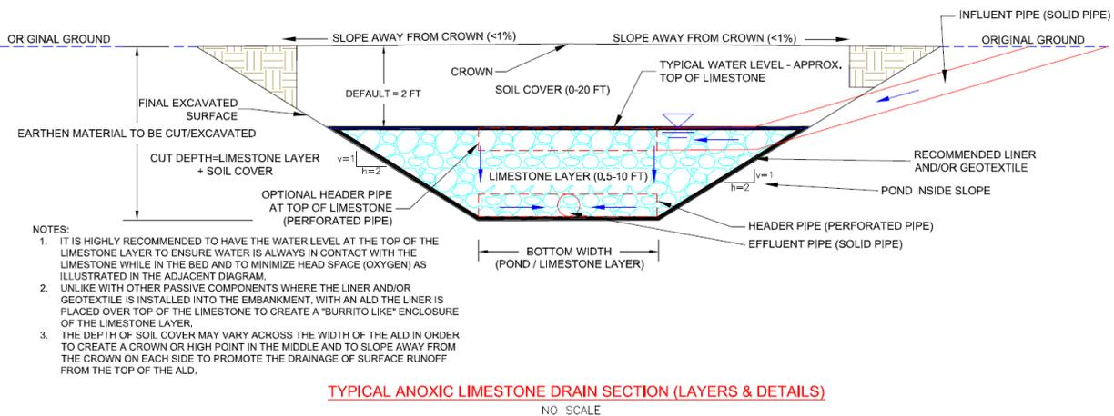
Figure 2: Typical Cross Section View of an Anoxic Limestone Drain (ALD) with a water layer.
