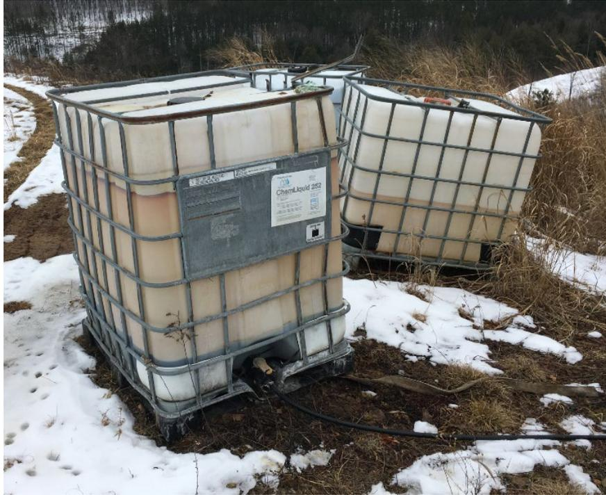
Figure 5: Picture of a 330-gallon tote of 25% Caustic Soda Solution being dosed from the 2-inch camlock valve assembly through poly feeder tubing. Note the reserve totes in the background.
