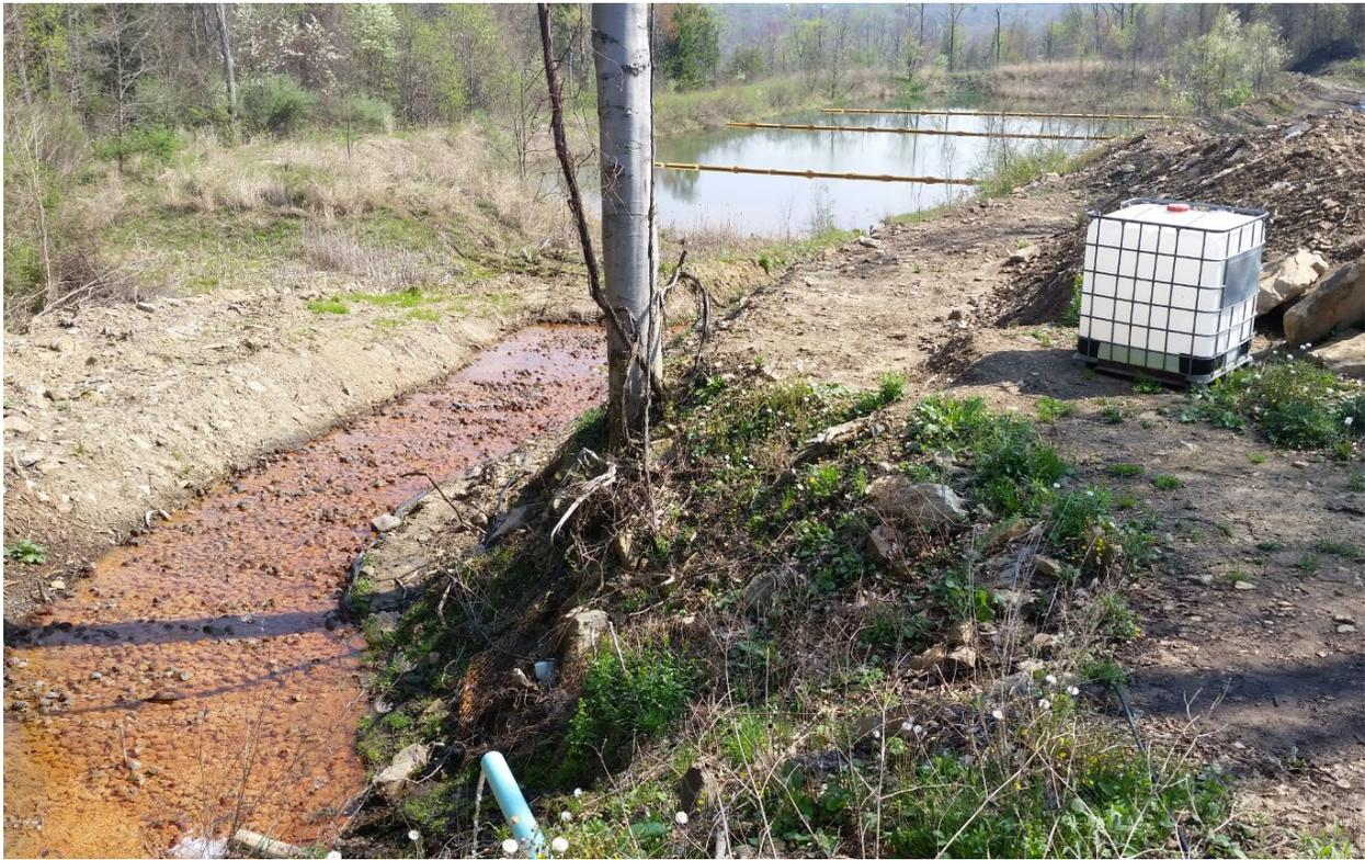
Figure 3: Caustic Soda being dispensed directly from a 330-gallon chemical storage tote. A poly feeder line and valve are attached to the tote for manual dosing.
