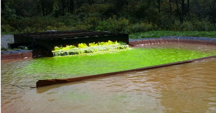
Figure 7: Dye testing on a Maelstrom Oxidizer decarbonation unit to determine the  $\text{CO}_2$  transfer coefficient.
