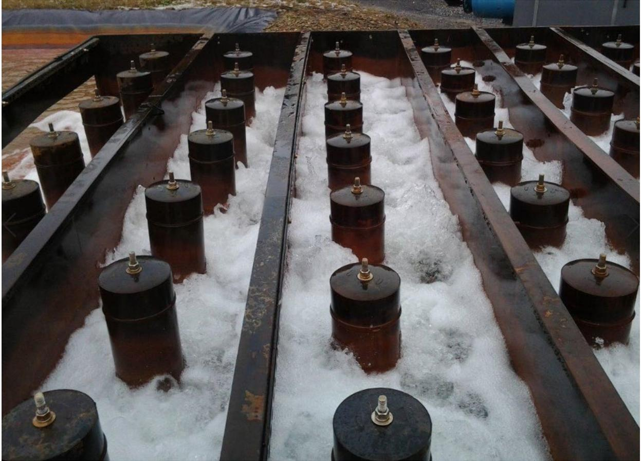
Figure 18: Maelstrom decarbonation tank showing vertical baffles separating the rows of air tubes.
