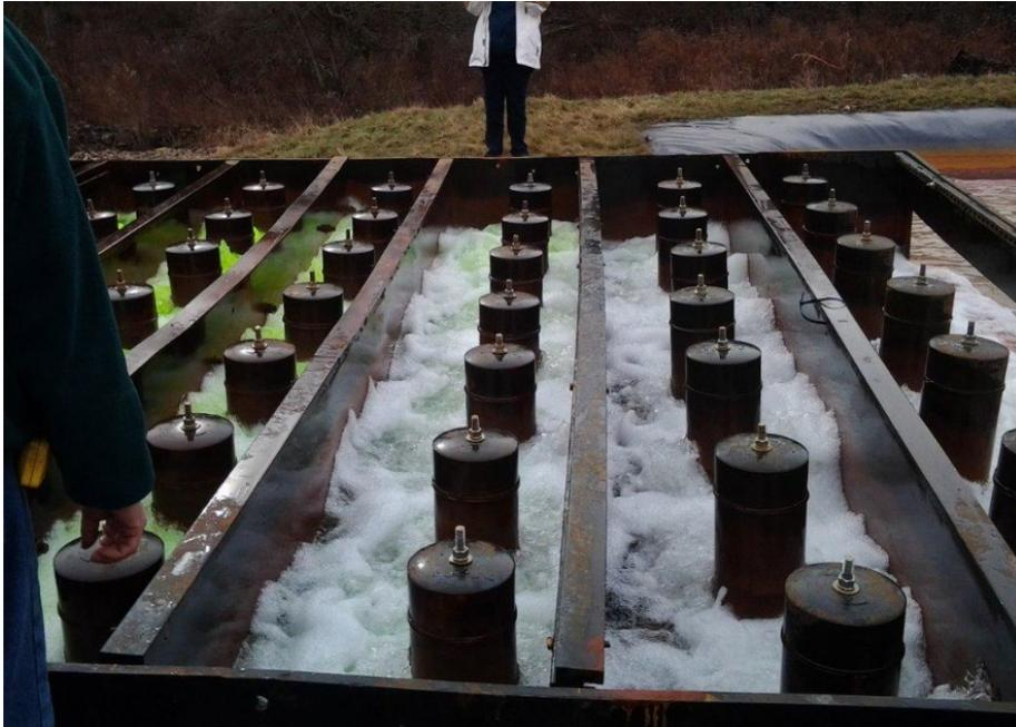
Figure 6: Dye testing on a decarbonation unit to determine the CO<sub>2</sub> transfer coefficient.
