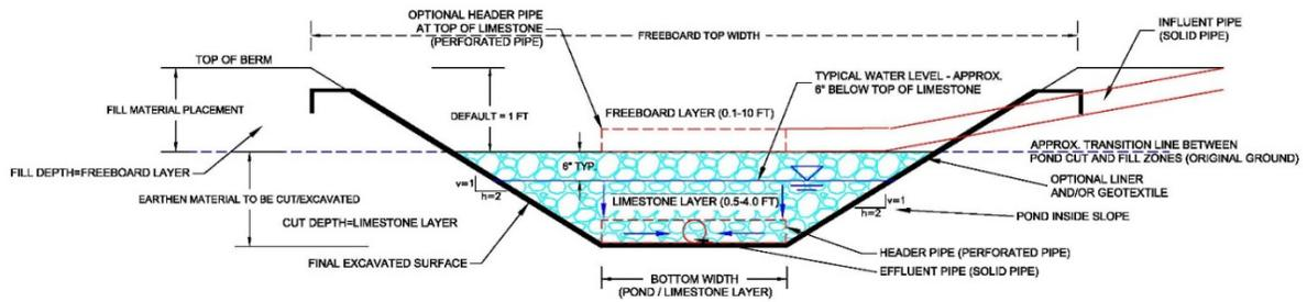
**TYPICAL MANGANESE REMOVAL BED SECTION (LAYERS & DETAILS)**
