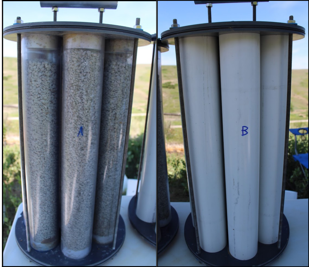
Figure 2.7: Assembled cartridges—A) clear PVC tubes filled with clinoptilolite, B) standard white PVC tubes.
