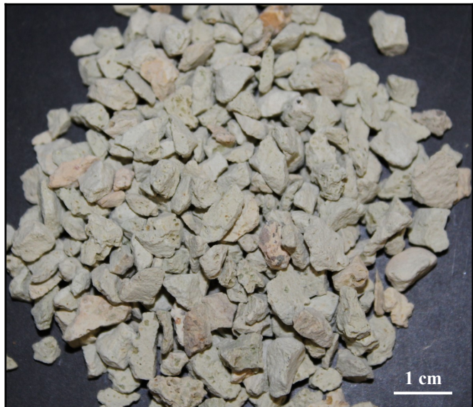
Figure 3.2: Clinoptilolite grains, 4 \times 8 mesh.
