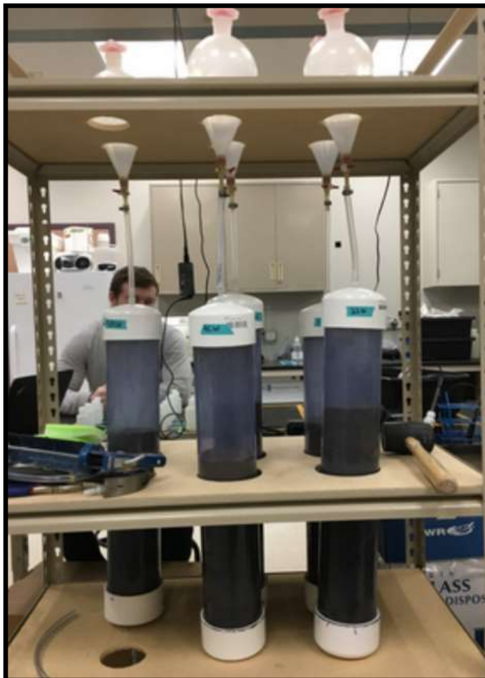
Figure 5. Constructed and filled leach columns for benchtop experiments conducted with Cordero Rojo Mine waste rock.
