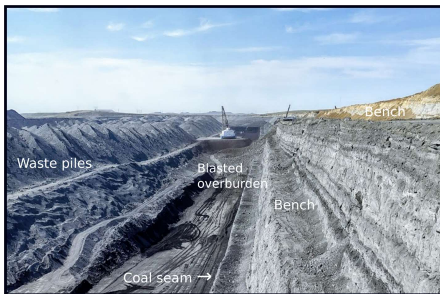
Figure 3. Example of the removal of overburden and waste generation during open-pit coal mining in a sedimentary basin, Cordero Rojo Mine, Powder River Basin, Wyoming, USA.
