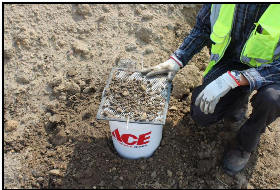
Figure 4. Cordero Rojo Mine waste rock samples being sieved to \leq 6.3 mm onsite.
