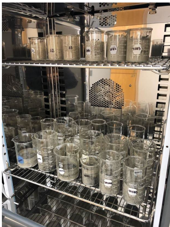
Figure 10. Collected samples were dried using a hot air oven.
