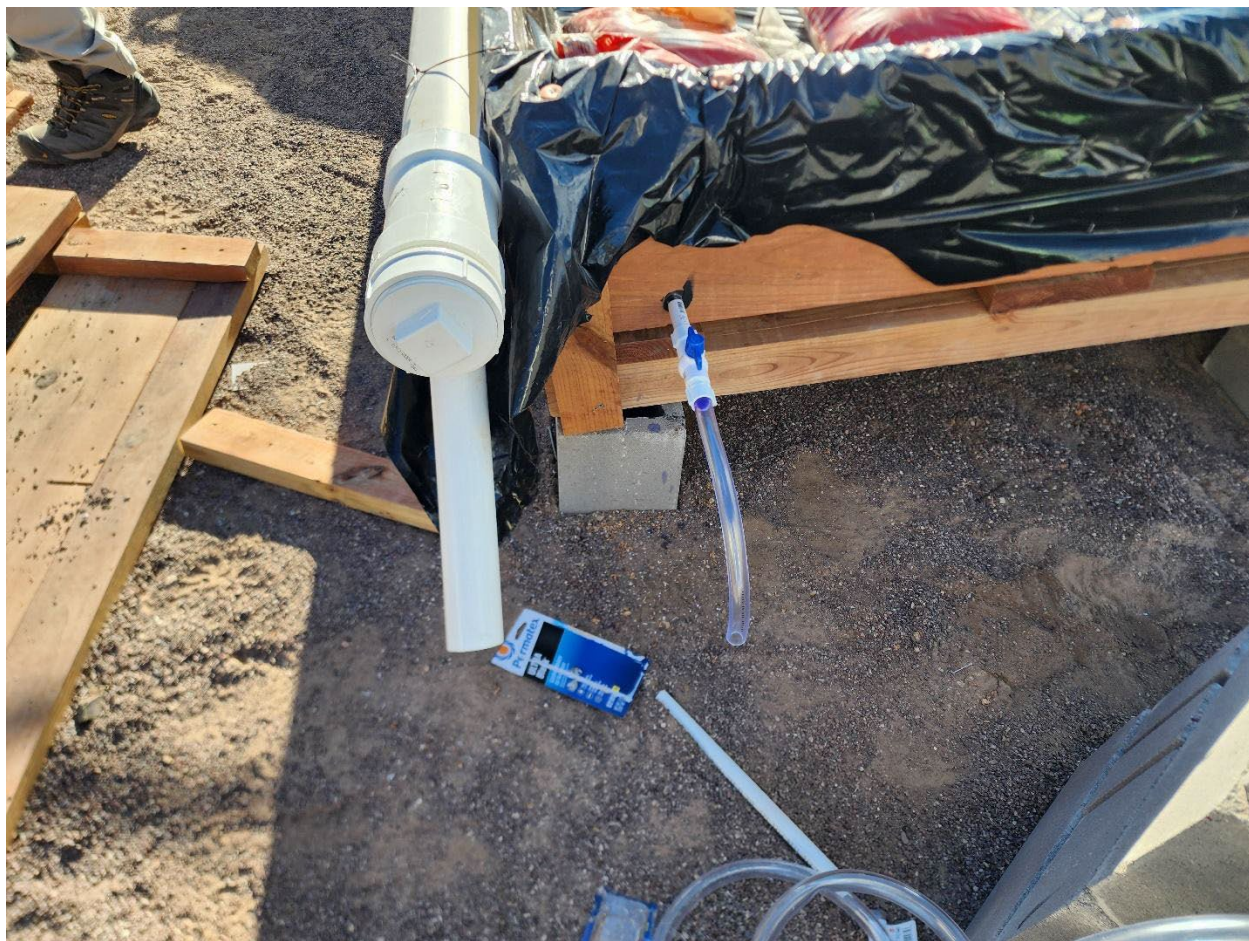
Figure 22. Each platform is equipped with leachate and surface run-off collection systems.
