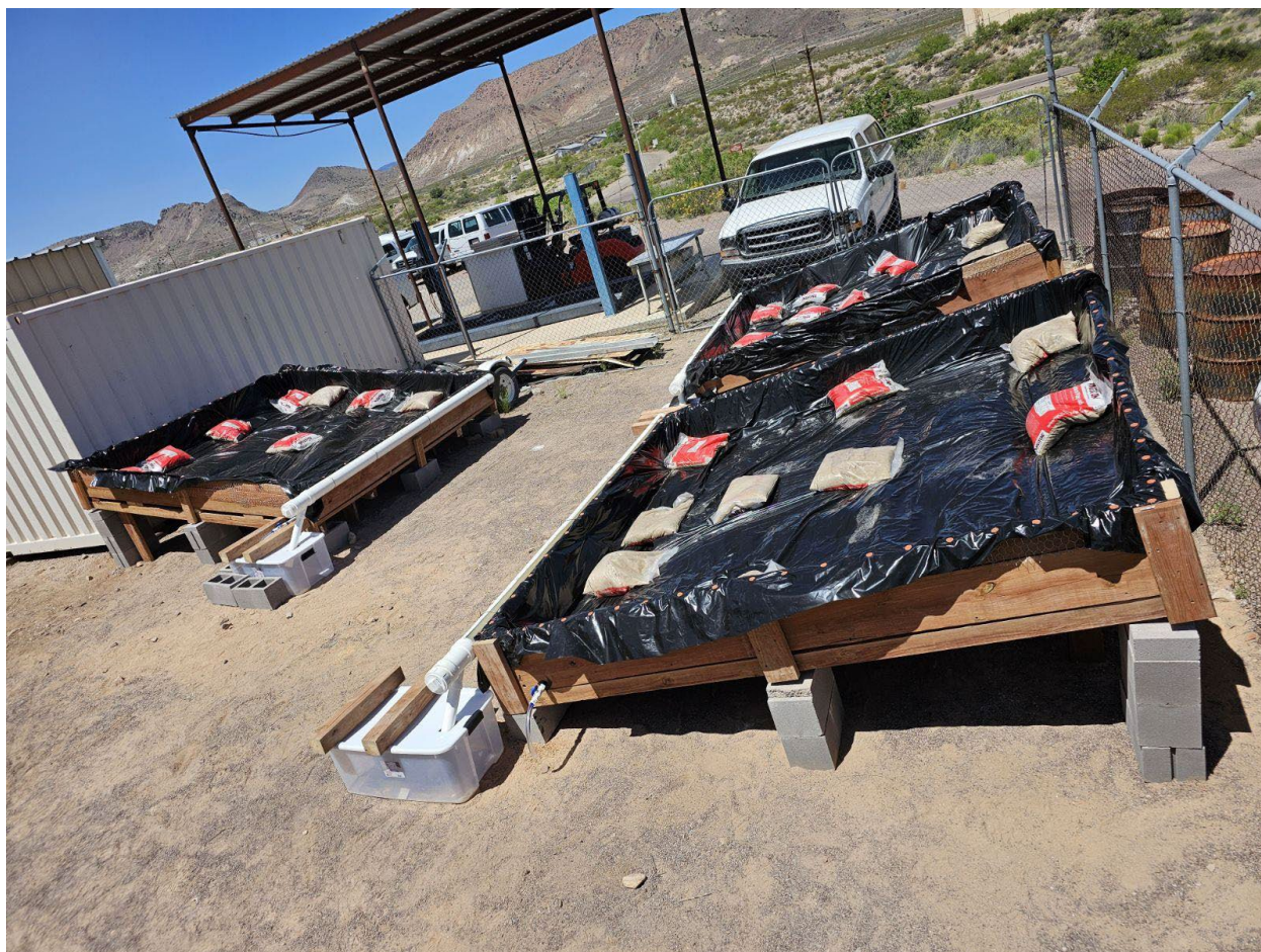
Figure 23. Three custom-made 10.0 ft. × 10.0 ft. × 1.0 ft. wooden platforms after complete assembly in Socorro.
