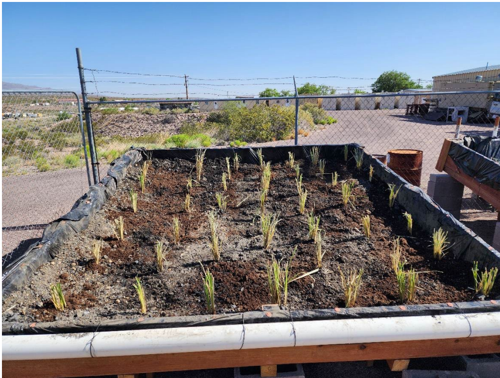
Figure 32. Vetiver panel with 49 vetivers planted in 7 rows.
