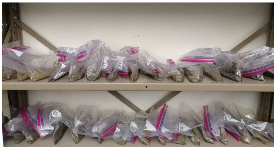
Figure 8. Soil Incubation Study at Navajo Technical University (NTU). A total of 30 bags containing compost and biochar amendments at different rates are being maintained at 70% of the soil water holding capacity. The incubation study will be conducted for 90 days.
