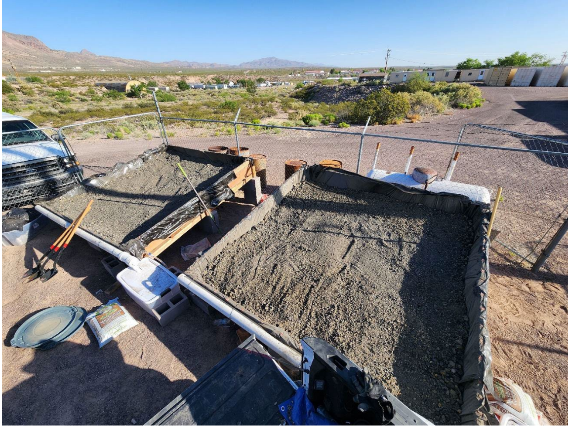
Figure 28. On top of the 5inches play sand 5inches of gob pile samples were dumped in each panel.
