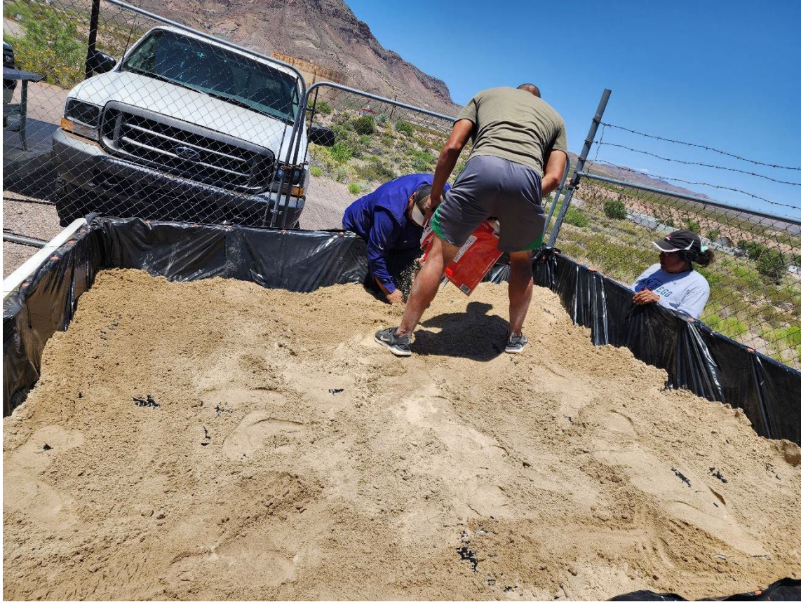
Figure 24. Each panel were loaded with 5inches of play sand in the bottom.
