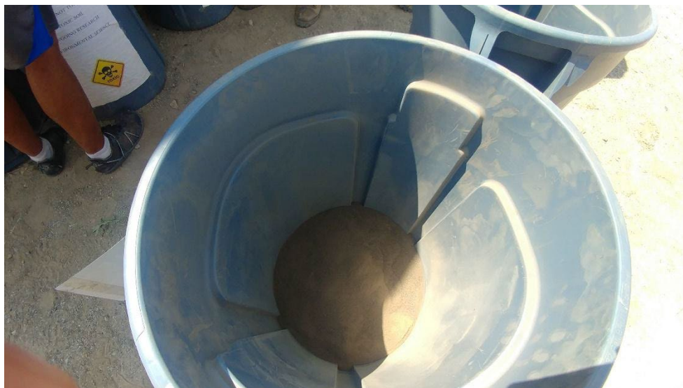
Figure 6: Carthage Coalfield (CCF) samples were air-dried, ground, sieved and stored until future use.
