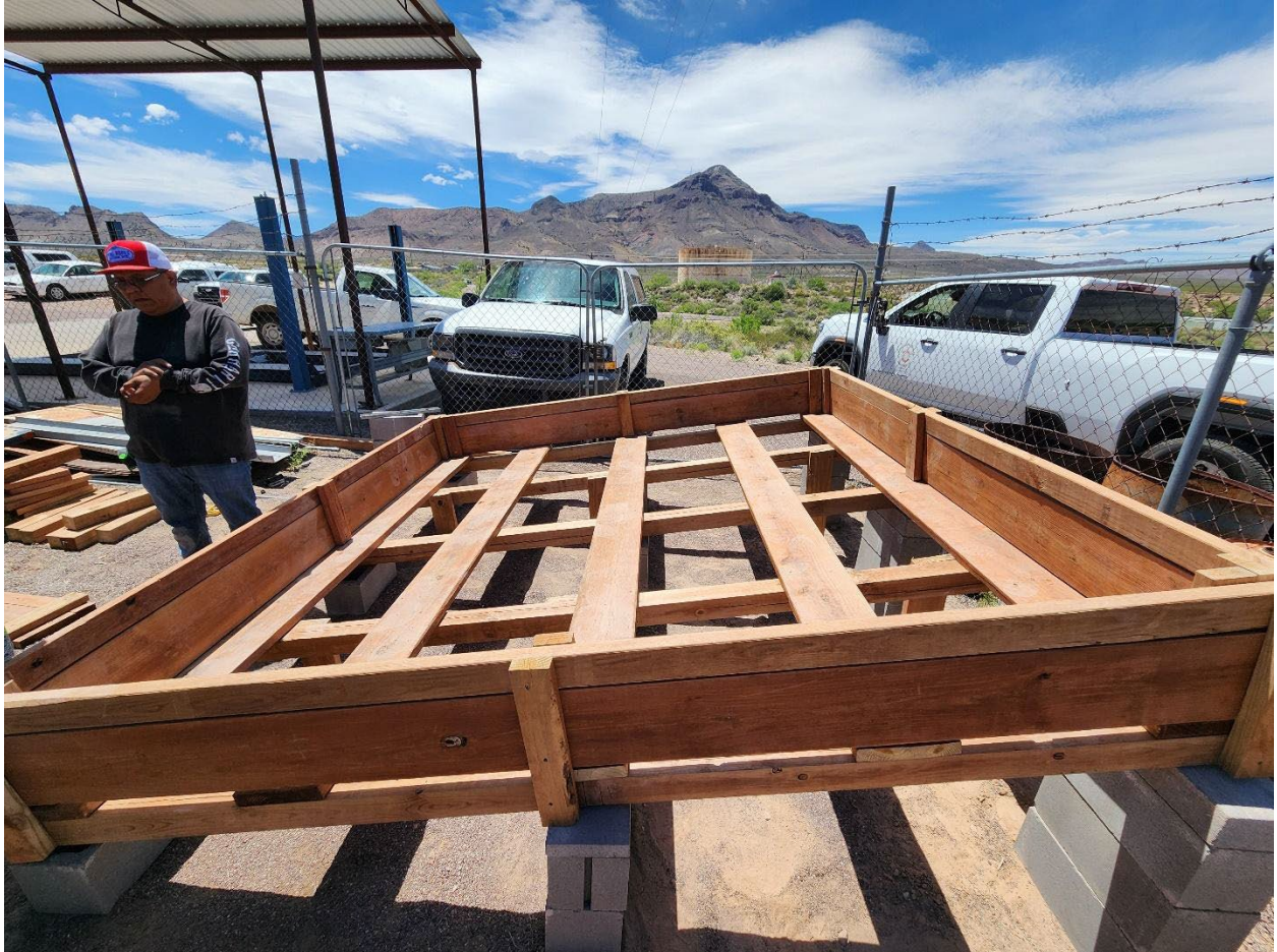
Figure 21. The slope of the wooden platforms was controlled by adjusting the panel leg heights with cinder blocks.
