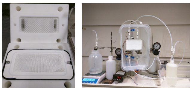
Figure 4. (Left) open CF042P cell showing a feed spacer (top) and permeate carrier (bottom); the outer edges of a flat membrane located underneath permeate carrier are also visible. (Right) MD setup showing a loaded cell with connections to peristaltic pumps and solution containers.
