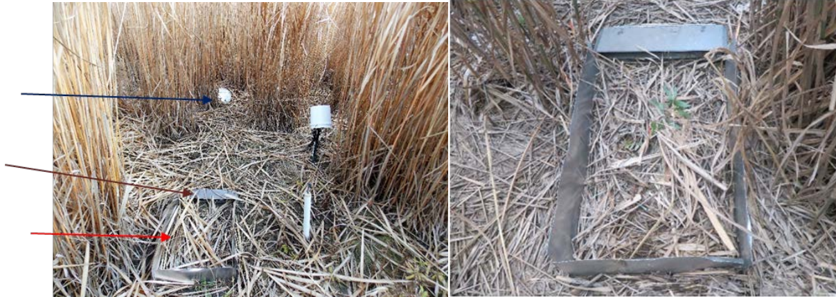
Photo 5. Left: Gerlach trough in a miscanthus plot for monitoring surface soil erosion and runoff water quality (Red arrow indicates runoff water collection area, brown arrow indicates location of Gerlach trough, blue arrow indicates where excess runoff is collected connected by a tube); Right: Detailed view of Gerlach trough in a miscanthus plot looking downslope (Photo credit: Jose Guzman).
