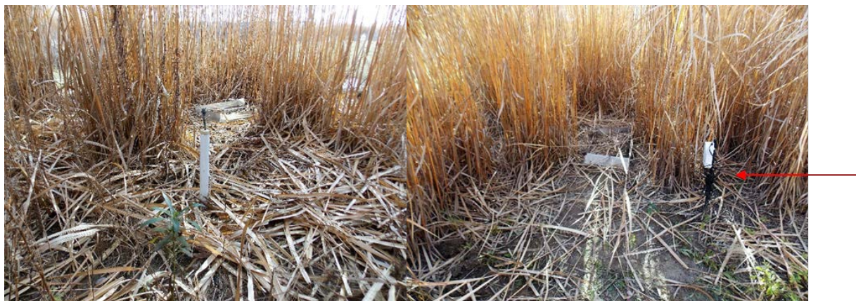
Photo 6. Left: Lysimeter in the middle of a miscanthus plot for collecting leachate at a depth of 25 cm (10 in) just below the root zone (Gerlach trough in the background); Right: Data logger (red arrow) in a miscanthus plot connected to soil temperature and moisture sensors inserted at soil depths of 5, 15, and 25 cm (2, 6 and 10 in) depth (Gerlach trough in the middle) (Photo credit: Jose Guzman).
