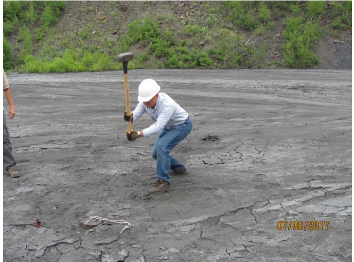
(b) Generation of shear waves by a sledge hammer
