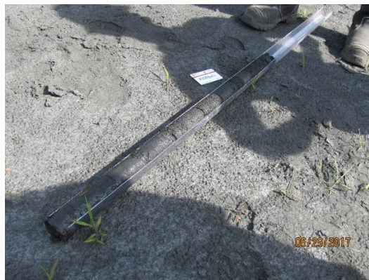
Figure 2-13. The retrieved fine coal refuse samples with PVC liners. Photos taken on 06/29/2017.
