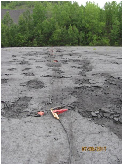
(a) Layout of a seismic line of 12 geophones
