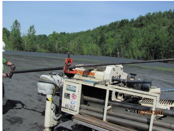
(b) sample retrieval and cutting
