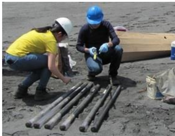
Figure 2-14. Labeling of the relatively undisturbed fine coal refuse samples
