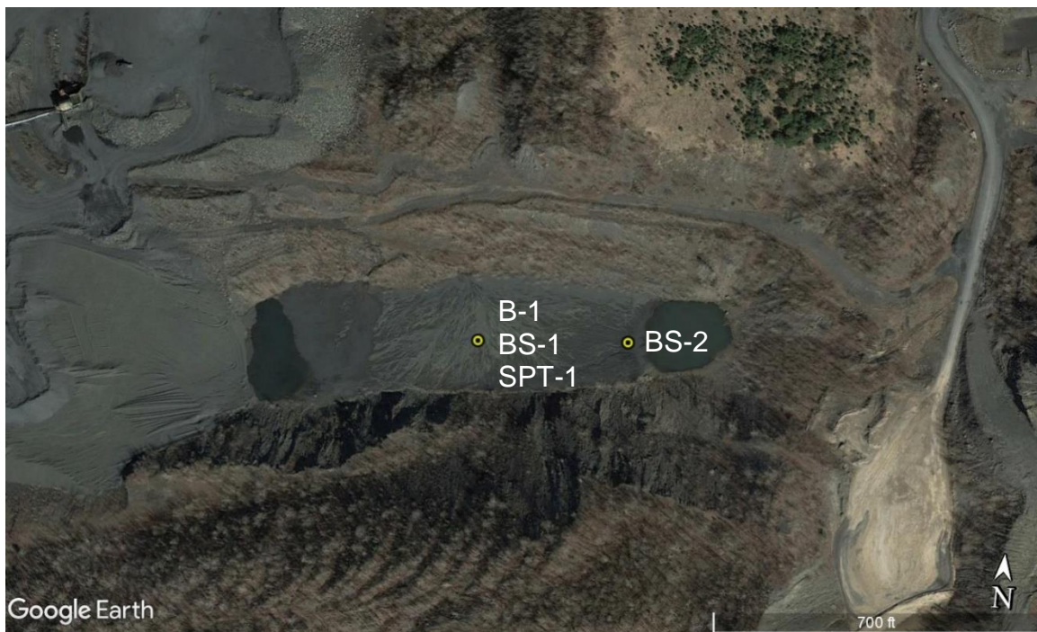
Figure 2-9. Layout of field testing and sampling at Site 2. Note: B-1, BS-1, and SPT-1 are at the approximately same location. “B” represents boring, and “BS” represents bulk sample.
