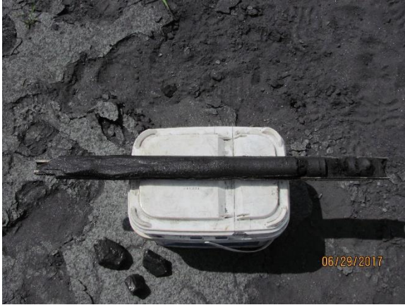
(a) The slurry-like fine coal refuse flowing out of the SPT split tube sampler
