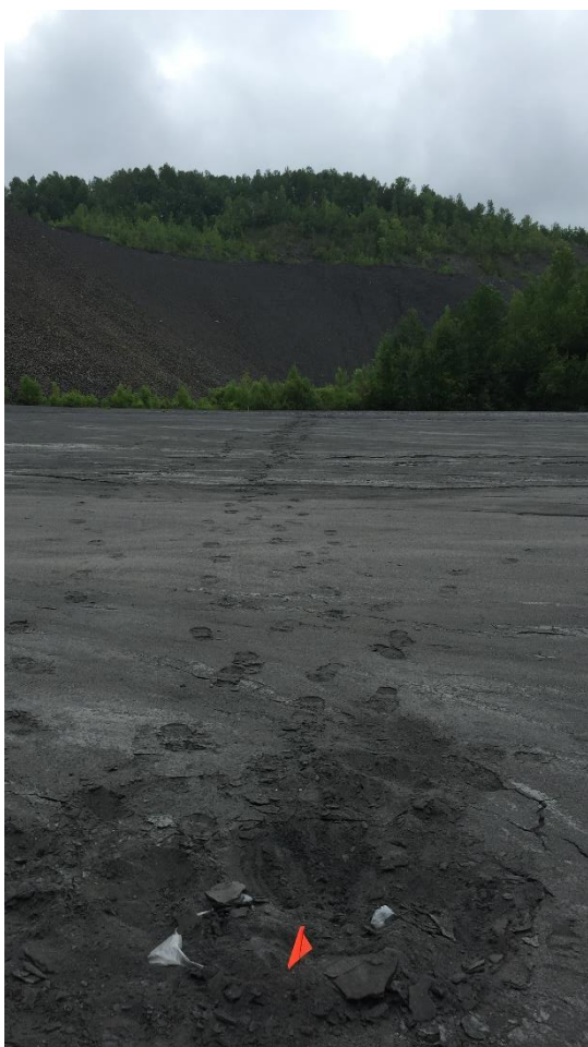
(a) A seismograph was buried 15 cm (6 inches) into the ground
