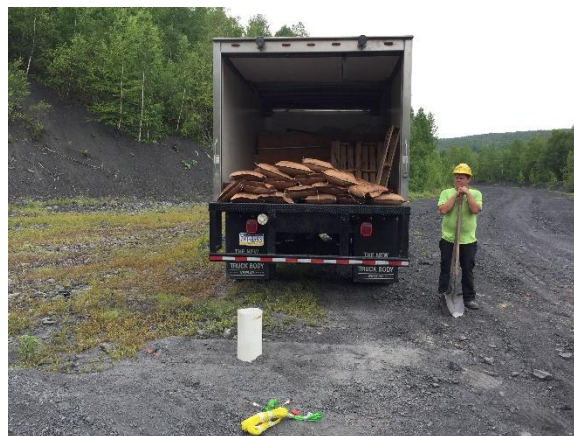
Figure 4-8. A blast hole for ground motion generation during the seismic monitoring on July 6, 2017
