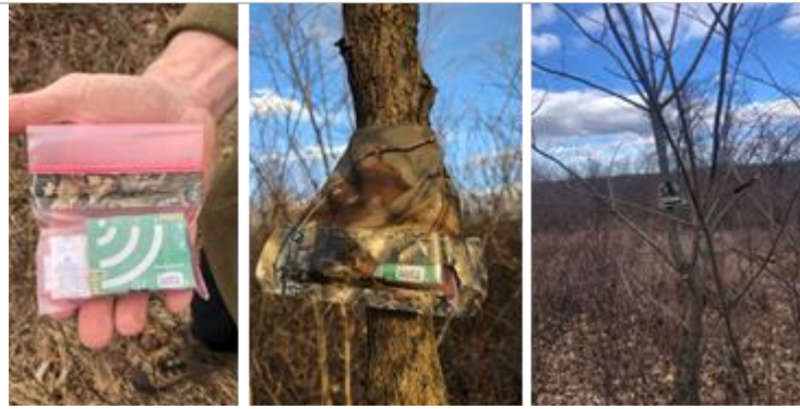
Figure I.1. Automated Recording Units (ARU) showing size and deployment. ARUs were used to monitoring birds, bats and amphibians are study sites.
