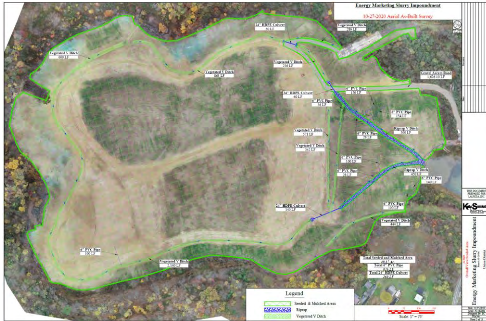
Figure 58. WVDEP reclaimed impoundment layout.
