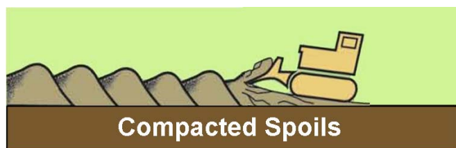
Diagram 3: The “Dozer Push-Up” method can be used to prepare uncompacted surfaces that are suitable for reforestation where materials for surface placement are moved over a short distance. Depending on the situation and State program policies, it may be possible to use the “dozer push-up” surface for reforestation without a final strike-off grading. Otherwise, the push-up piles should be struck off with one or, at most, two passes with a light dozer.
