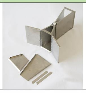
**Description:** This stainless steel, flat-bottom flume can be disassembled for easy transport. It can be set up with either a one-inch throat (2.5–125 gpm) or four-inch throat (10–250 gpm). The unit comes with entrance wing walls to divert flow into the upstream converging section of the flume.
