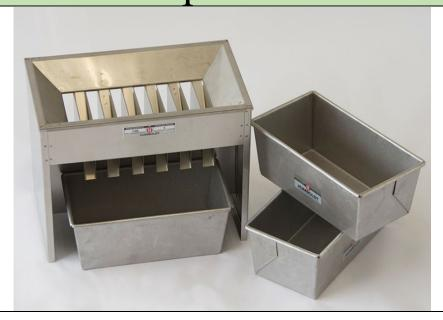
**Description:** This 14-inch-long stainless-steel sample splitter has a removable hopper constructed of 12 chutes that discharge alternately to front and back. Chutes are <sup>3</sup>/<sub>4</sub> inch wide. Two pairs of cold-rolled steel pans come with the unit.
