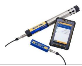
**Description:** The AquaTROLL 500 MP handheld instrument has a combined pH/ORP sensor and other sensors for temperature, conductivity, pressure, and dissolved oxygen. The completely submersible sensor-equipped probe is connected to the rechargeable power pack. Sensor readings are transmitted by Bluetooth from the power pack to the Android or iOS tablet/smart phone. The unit uses In-Situ's VuSitu app to collect the data.
