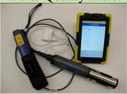
**Description:** The smarTROLL MP handheld instrument has a combined pH/ORP sensor and other sensors for temperature, conductivity, pressure, and dissolved oxygen.
