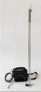
**Description:** The Marsh-McBirney Model 2000 Flo-Mate uses an electromagnetic sensor to measure water velocity. Powered by two D-size batteries, the unit has a measurement range of -0.5 to +19.99 feet per second (-0.15 to +6 meters per second). The top-setting wading rod allows the sensor to be conveniently set at 20%, 60%, and 80% of total depth.
