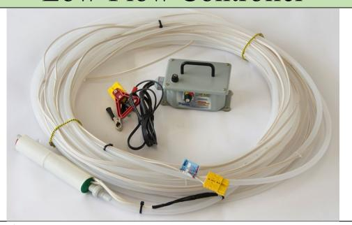
**Description:** Mega-Typhoon is a 12 VDC two-stage submersible pump that has 80 feet of 3/8-inch ID HDPE tubing (tubing volume is 0.6 gal). The plastic pump body measures 1.7-inch OD by 10-inch length. Used with the Low Flow with Power Booster 1 controller, the pump will produce 3.5 gpm at 10 feet of head and 0.25 gpm at 80 of head.
