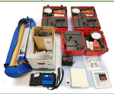
**<u>Description</u>**: The Leica RTK 500 GPS survey system is a high-accuracy GPS/GNSS system for field surveying and data/point collection. The system consists of:
