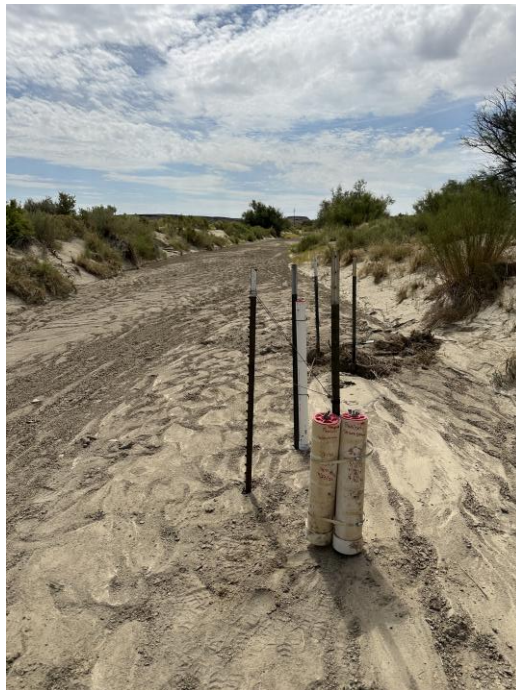
Photo 2 Surface water samplers located in Pinabete Arroyo, referred to as “Lower Pinabete”
