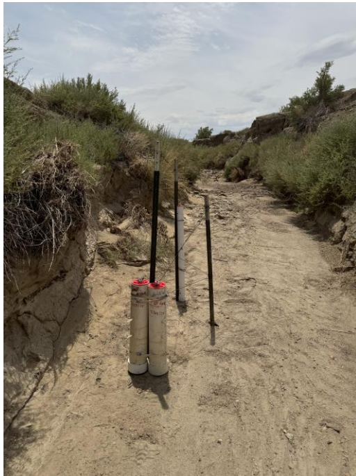
Photo 4 Surface water samplers located in No Name Arroyo, referred to as “Lower No Name”
