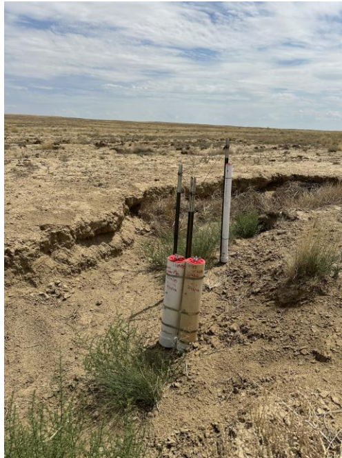
Photo 3 Surface water samplers located in No Name Arroyo, referred to as “Upper No Name”
