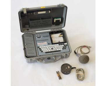
**Description:** The portable seismograph system—usually set up at a house—records ground vibration and sound (airblast) from blasting events. The seismograph system includes:
