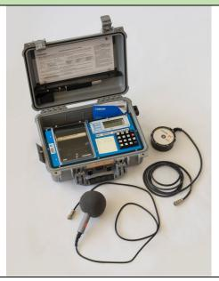
**Description:** The portable seismograph system—usually set up at a house-- records ground vibration and sound (airblast) from blasting events. The seismograph system includes:
