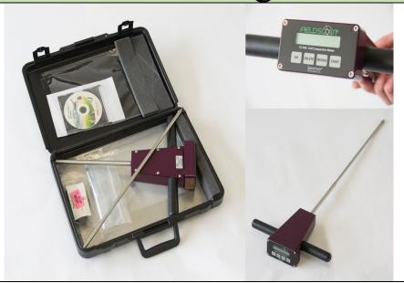
**Description:** The portable soil compaction meter uses a cone penetrometer to measure soil compaction to a depth of 18 inches. The unit has a datalogger function that allows measurements to be downloaded to a computer. The unit can also log GPS location using a Bluetooth connection to an appropriate GPS unit.
