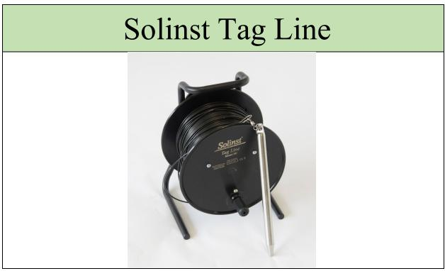
**Description:** This tag line has a 500-foot polyethylene coated, permanently marked stainless steel cable clipped to a <sup>3</sup>/<sub>4</sub>-inch stainless steel weigh. The tag line is wound on a 10-inch diameter plastic reel with a brake. Every foot is labeled, and additional cable markings are at every <sup>1</sup>/<sub>4</sub> foot.
