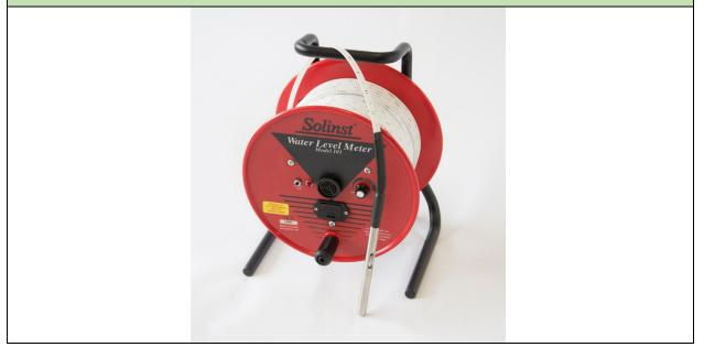
**Description:** The water-sensing probe is attached to a 300-foot polyethylene flat tape with permanent markings every 1/100 of a foot. A dial allows the buzzer to be adjusted or turned off when the probe is in cascading water and ensures a clear signal when the probe contacts high- or low-conductivity water. The tape is wound on a 10-inch diameter plastic reel with a brake.
