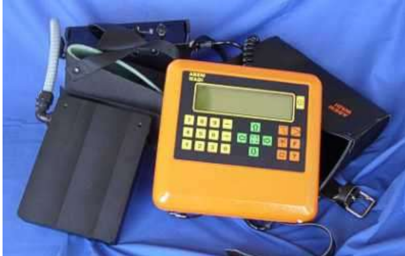
Figure 20. Picture of ABEM-Wadi VLF Instrument, similar to the one used to collect mid-depth electromagnetic anomalies along stream profiles.
