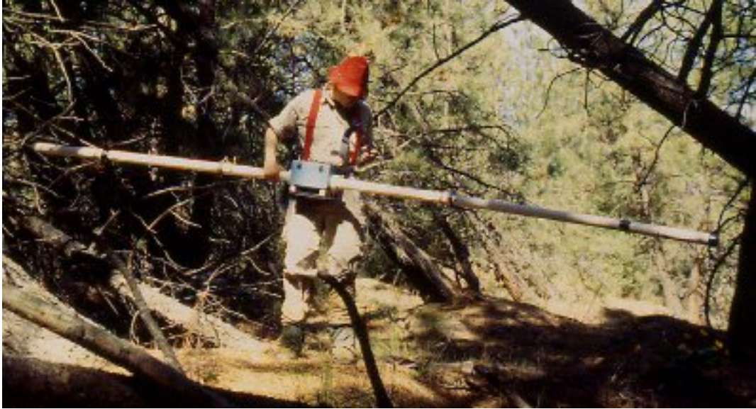
Figure 17. Example picture of Geonics EM-31 Terrain Conductivity meter.
