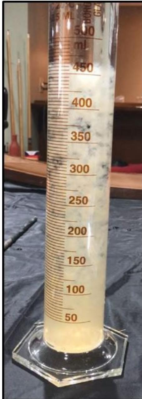
Figure 1: Settling test determining the settling rate for a specific concentration of flocculated aluminum hydroxide produced solids.
