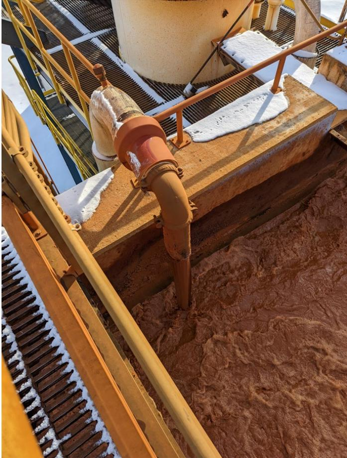
Figure 29: Example of an Enhanced Flocculation treatment system. Sludge from the clarifier is pumped back into the reaction tank where it is mixed with mine water treated with hydrogen peroxide. The pipe is recirculating approximately 250 gpm of 4% solids by weight back to the reaction tank.
