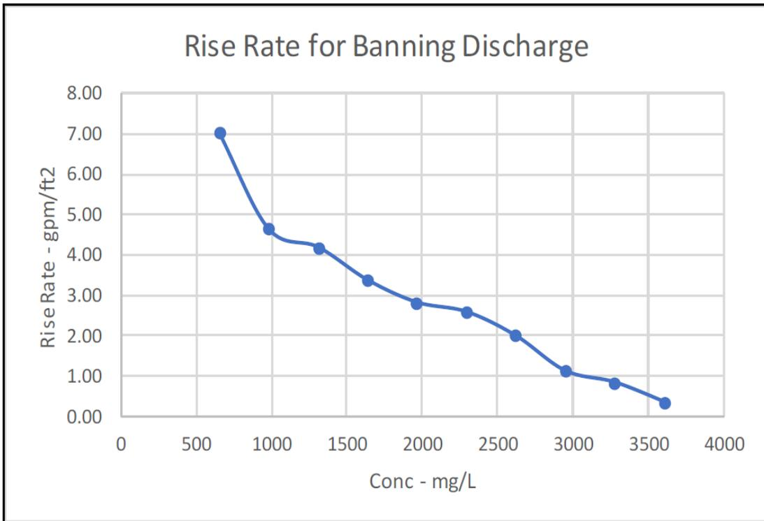
Figure 2: Results of ten settling tests to relate the rise rate to the concentration of produced solids.
