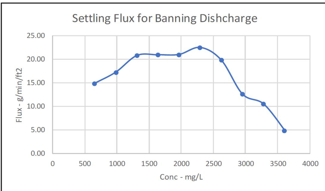
Figure 3: The settling flux rate characterizes the optimal solids loading.
