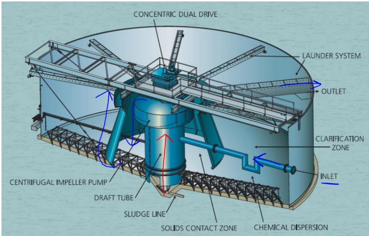
Figure 20: Schematic of a Solids Contact Clarifier (courtesy of Westech Engineering). Blue arrows signify the flow of water and the red arrow indicates how the sludge is pulled back to the surface to mix with raw water.
