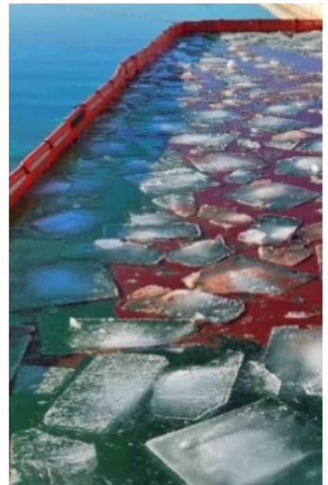
Oil flows through a simulated ice field formed from the manufactured ice.
