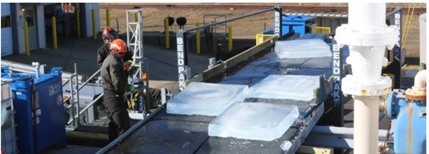
New ice-making capabilities at Ohmsett provide a method to create reproducible ice fields that simulate arctic conditions. In this photo, ice blocks slide down the lifting system and into the tank.
