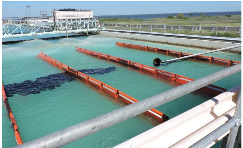
Booms and water management tools allow for testing of multiple oils on the tank simultaneously.
